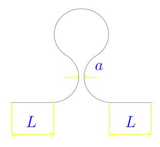
If  $\Gamma$  is a straight line, the transverse eigenfunction is  $\mathrm{e}^{-\alpha|y|/2}$ , hence the distance at which tunneling becomes significant is  $\approx 4\alpha^{-1}$ . In the example, we choose  $\alpha=1$
