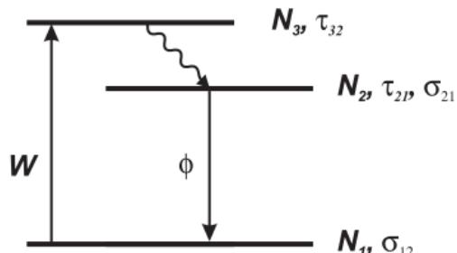
$$\begin{aligned}\frac{dN_3}{dt} &= W - \frac{N_3}{\tau_{32}} \\ \frac{dN_2}{dt} &= \frac{N_3}{\tau_{32}} - \frac{N_2}{\tau_{21}} - \sigma_{21}c\phi N_2 + \sigma_{12}c\phi N_1 \\ \frac{dN_1}{dt} &= -W + \frac{N_2}{\tau_{21}} + \sigma_{21}c\phi N_2 - \sigma_{12}c\phi N_1\end{aligned}$$
