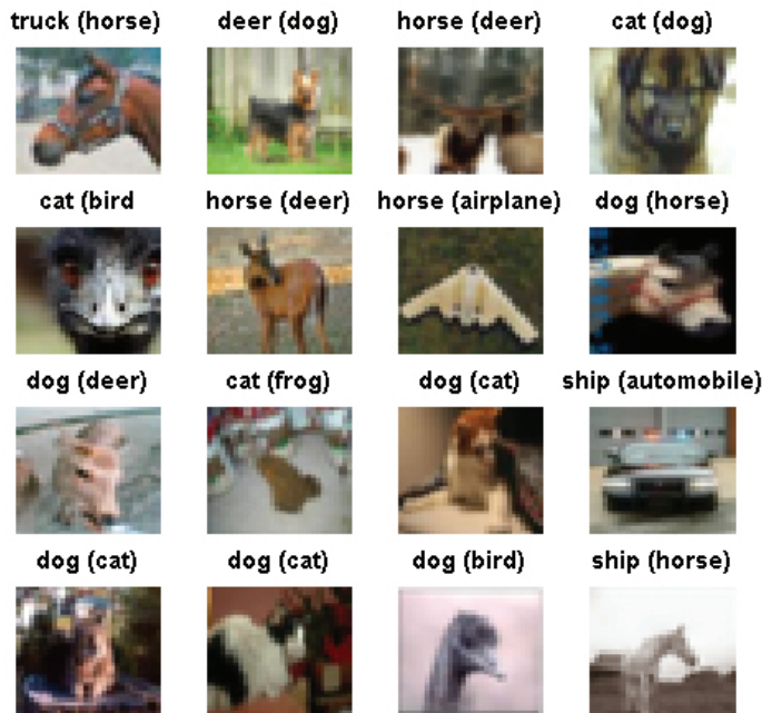
Fig. 7.6 Sixteen of the images that were misclassified by the trained network from Figure 7.2. The predicted category is indicated, with the correct category shown in parentheses. Note that images are low resolution, with 32 \times 32 pixels.
