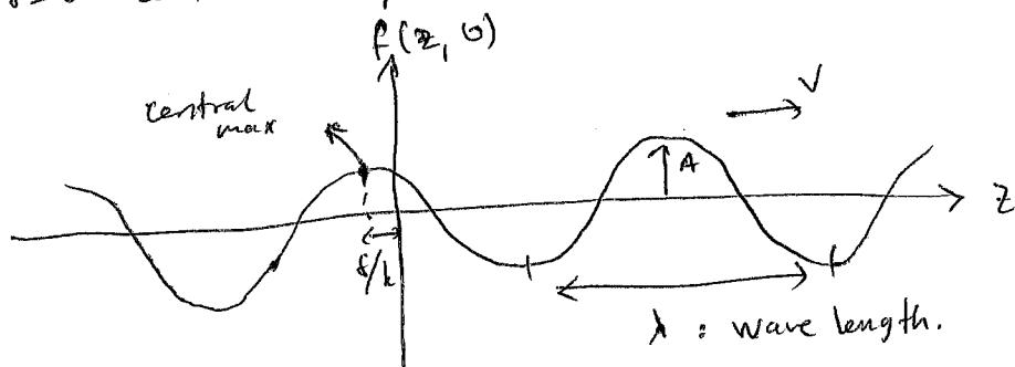
$$k = \frac{2\pi}{\lambda} \quad \begin{matrix} \text{wave number} \\ \text{wavenumber} \end{matrix} \quad \left. \begin{matrix} \text{If } z \text{ advances } \frac{2\pi}{k} \text{ cosine completes a cycle.} \end{matrix} \right\}$$
