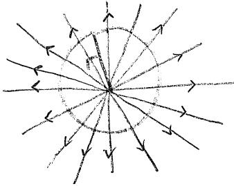
$\frac{n}{2\pi r}$  : # of field lines divided by the circumference of a circle } line density goes like with radius  $r$  }  $1/r$ , not  $1/r^2$ .
